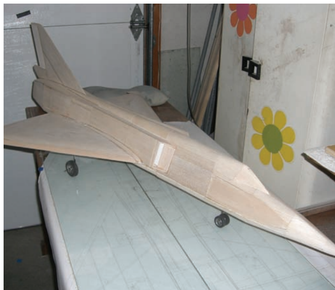
The only thing left is to shape the nose block, rudder fairing block and rudder, then glue them to the fuselage and it's time for final finishing and my favorite part—flying!
