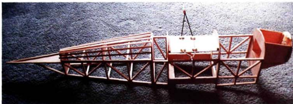
The fuselage has been framed except for the belly and nose bottom. Build the nose cone separately and add it later.
