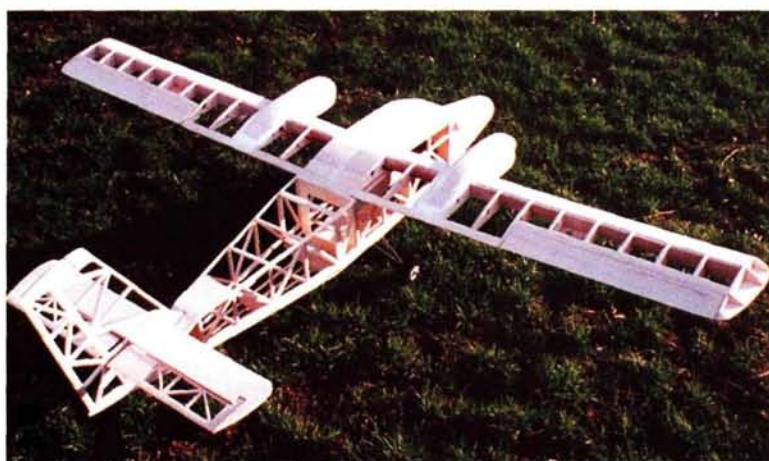
Here's the Twin Otter, built and ready to cover. Note that the stabilizer should be open frame and not sheeted as shown here. Just follow the plan.
