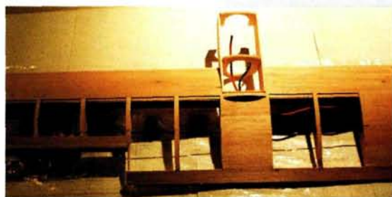
This view of the top of the left wing shows the nacelle during construction. The formers are in place and are ready to be sheeted.
