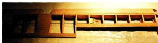
Here's the right wing panel minus the motor nacelle. Note the simple aileron bell-crank and pushrod system.
