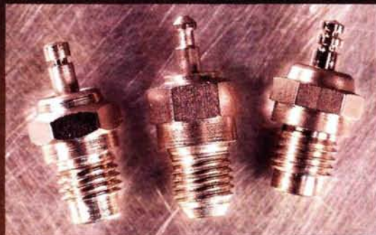
Special glow plugs for 4-stroke engines (left to right): the O.S.-F plug is the granddaddy of all 4-stroke glow plugs and the originator of the extended-nose concept of temperature retention; the Merlin "Hosenose" plug incorporates interesting internal cavity dimensions and element design; Enya's latest entry features traditional technology.
