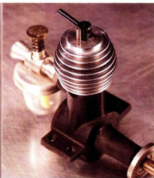
Turning the compression adjustment lever clockwise (as viewed from the top) increases this model diesel engine's compression ratio; turning it counterclockwise lowers the compression.
