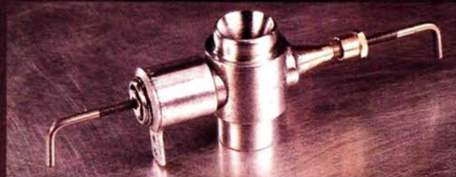
Above: this Super Tigre fuel-metering (twin-needle valve) carburetor illustrates a major technical advance in controlling the engine's air/fuel mixture during idle and throttle-up during the 1960s. Despite improvements in carburetion, crankcase-loading and plug-element-quenching continue to plague RC engines.
