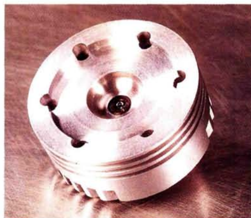
With the cylinder head removed from the engine, the long-reach standard glow plug should be flush with the upper surface of the combustion chamber (as shown).
