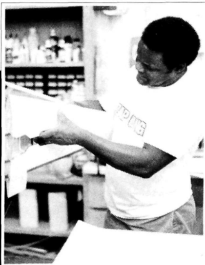
1. Sand the structure very carefully. Glass-cloth is so fine that any little protrusions will snag it and cause it to run—just like a nylon stocking.
