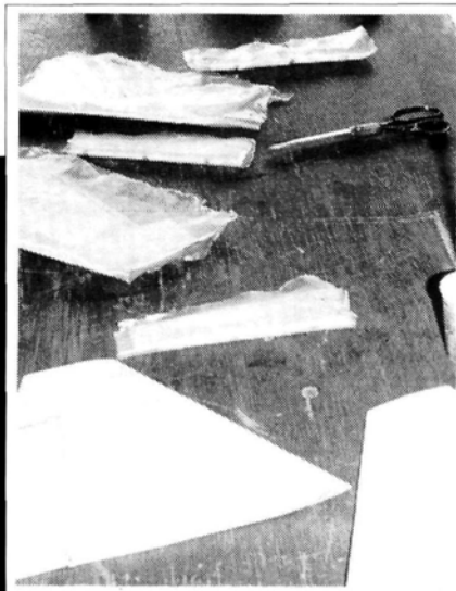
2. The cloth is cut slightly oversize and laid over the parts that will be covered. (Sharp scissors are a must!) You can use either polyester or epoxy resins and achieve good results.
