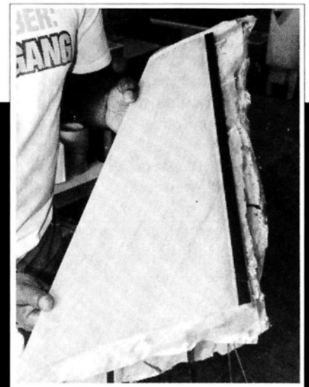
6. Here's a finished wing panel. After the resin cures for a few hours, the extra cloth is cut and sanded.
