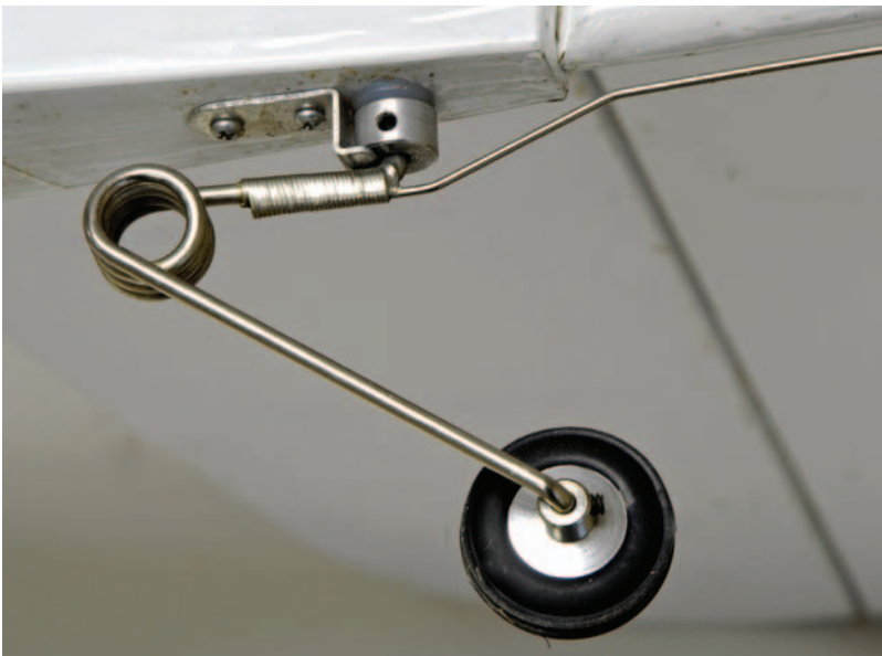
This tailwheel is supplied with the Great Planes CAP 232 and the Super Sportster ARF kits and is also available separately. It's light and easy to install.
