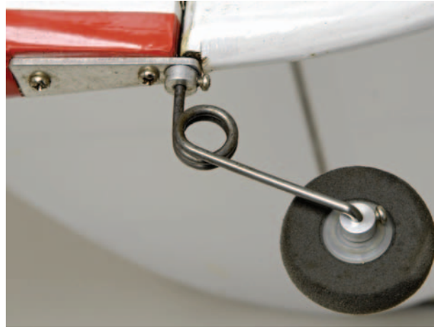
Left: This Sullivan Products tailwheel assembly is one of the best I've used for sport airplanes. It is available in four sizes; choose one to suit your model's weight. Right: This tailwheel is typical of what you find in most ARF kits. It looks strong but does not prevent steering shock from reaching the rudder servo.
