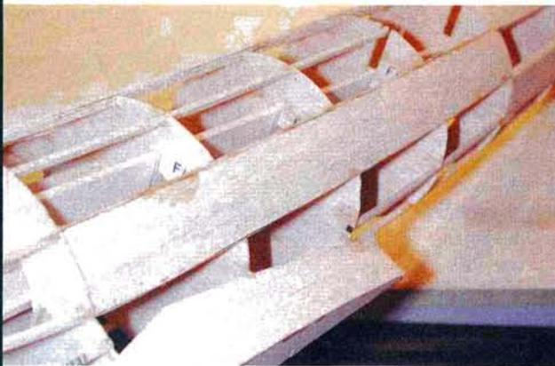
Attach the outer sheeting to the fuselage in sections, as shown here. The crutch has been removed from the fuselage. When the fuselage is rigid enough to hold its shape, remove the internal crutch and add the rest of the sheeting.
