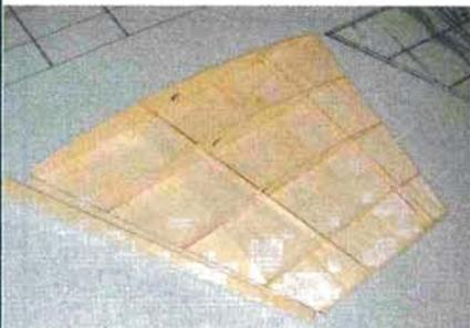
The basic wing structure is very simple. The ribs are glued on top of the bottom sheeting.
