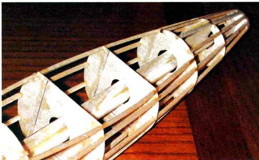
Here, the fuselage is taking shape, and several stringers have been installed. Notice the alignment crutch that runs through the formers. It will be removed later.
