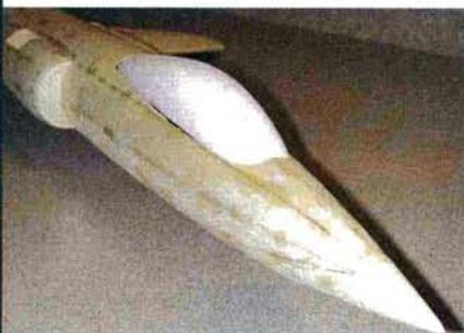
The nose cone and foam canopy add the finishing touches to the fuselage.
