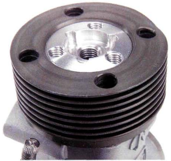
The cylinder head has a unique multipiece design. The three tapered holes in the central ring are for setscrews that provide additional support of the combustion chamber when high-nitro fuel is used.
