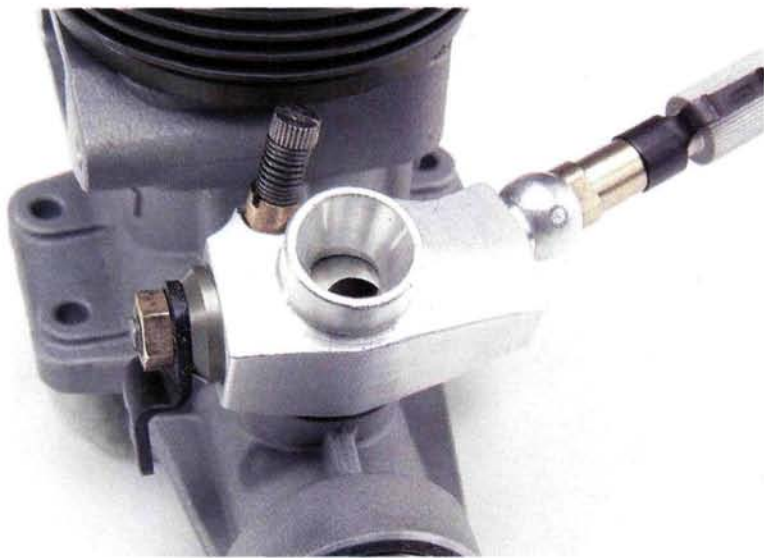
The 2-needle carburetor has a unique shape that slants the main needle valve aft and away from the prop.
