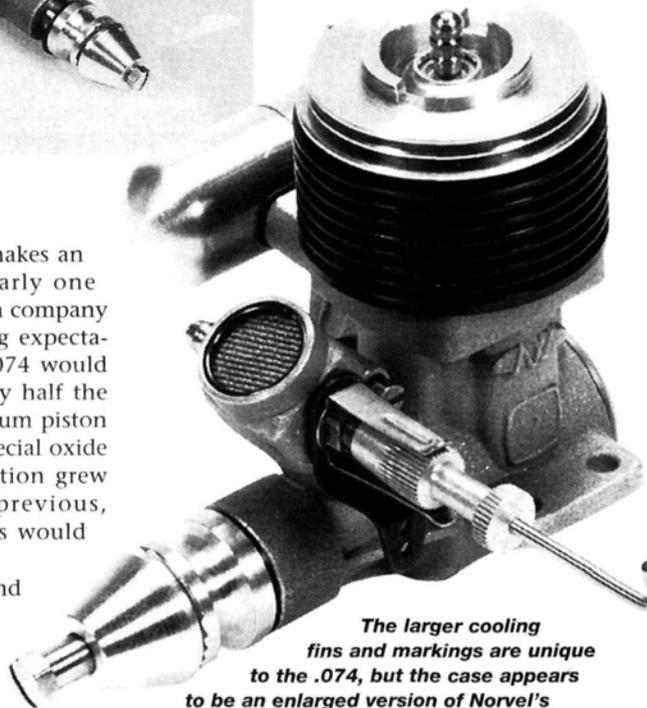
The larger cooling fins and markings are unique to the .074, but the case appears to be an enlarged version of Norvel's popular .061. By removing the nut just below the fuel intake, the carburetor can be rotated 180 degrees.
