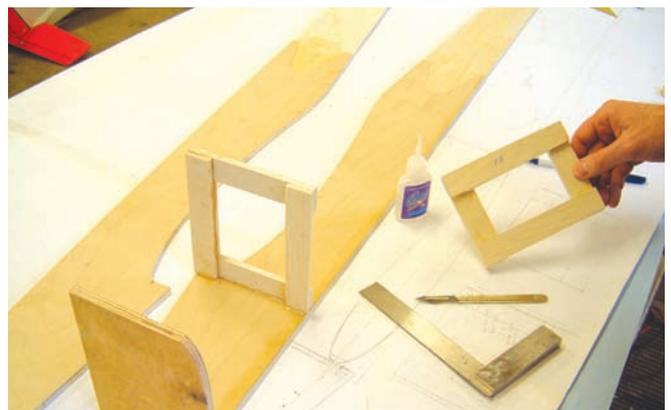
The ply firewall and two built-up balsa formers are shown glued to one side.
