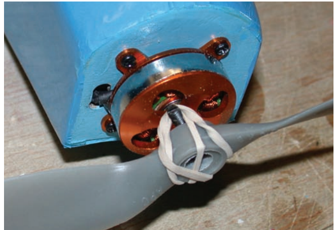
BP Hobbies Gold 2204-19 brushless outrunner motor is reliable yet very inexpensive. The prop is an APC 8x3.8 Slow-Flyer type.
