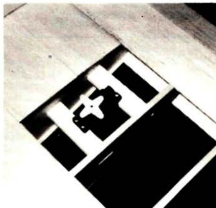
Individual aileron servos for slop-free setup, necessary in high-performance airplanes.
