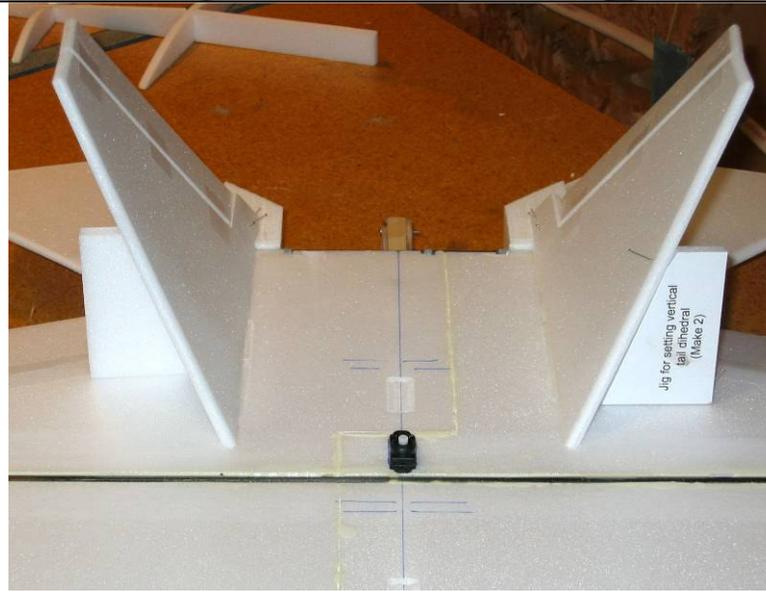
**16.** Sand the leading edge of the vertical tails to a well-rounded shape, and sand the trailing edges to a tapered shape. Apply a strip of 3M Gift tape to the leading edge.
