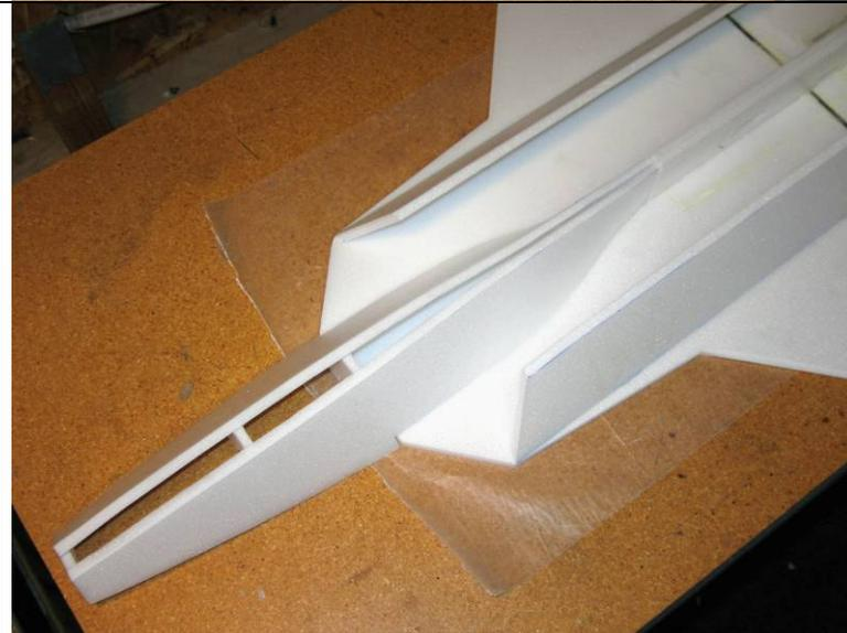
5. Glue the forward fuselage lower assembly in place on the front of the wing. Make sure the aft end of the forward fuselage mates with the forward edge of the centerline support piece. Also make sure the curvature is smooth as the angled forward fuselage sides twist to meet the vertical centerline support. Some trimming and additional heat-forming will likely be required to get a smooth curve here.
