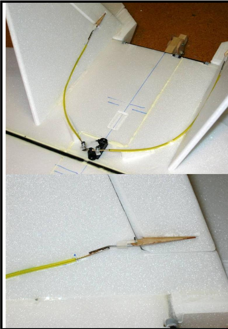
**17.** If incorporating rudders, install the control hardware now. Rudders are not required, but are helpful for improved control at high alpha and for better aerobatics.
