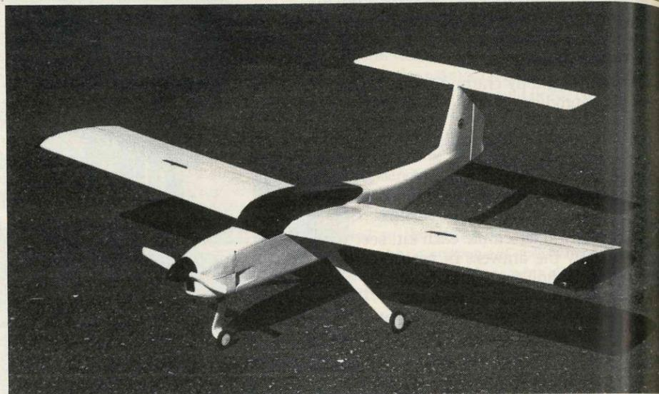
Crane II proved highly successful in flight and provided a great deal of insight into slotted wings and stabilator, variable pitch props, control spoilers, and flaps.
