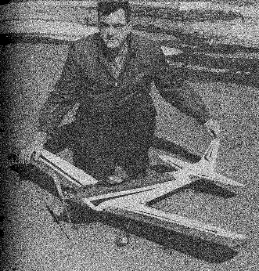
Smaller, lighter, cleaner, Ed's Orion replaces modified "Astro" he flew last year. Important feature is balancing of aileron effect to eliminate yaw. High stab gets away from downwash.
