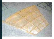
The basic wing structure is very simple. The ribs are glued on top of the bottom sheeting.
