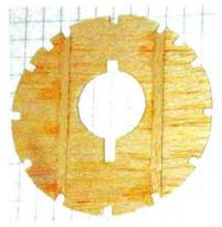
Start by cutting out all the formers. To avoid tearing away the corners, cut the notches out first and then cut out the rest of the former.
