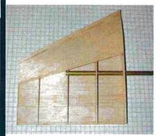
The main wing spar is a brass tube that plugs into the fuselage.
