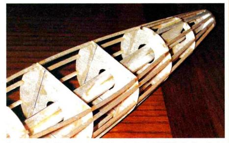
Here, the fuselage is taking shape, and several stringers have been installed. Notice the alignment crutch that runs through the formers. It will be removed later.
