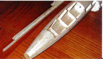
Attach the outer sheeting to the fuselage in sections, as shown here. When the fuselage is rigid enough to hold its shape, remove the internal crutch and add the rest of the sheeting.
