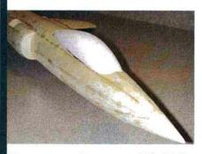
The nose cone and foam canopy add the finishing touches to the fuselage.
