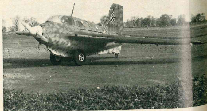
Front view shows the clean cowling of the engine, also belly skid.
