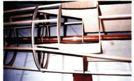
Left: start building the fuselage by assembling the main box structure. Note the temporary brace, FXX, tack-glued inside the box; it holds the structure in alignment on the jig tube. Right: the copper jig tube has been inserted through the circular formers. Below: after sliding the formers onto the tube, add the stringers. Alternate sides to keep the structure straight.
