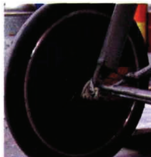
Landing-gear detail. Note the functional bungee shock cords.
