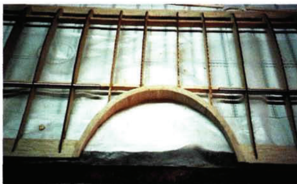
The top wing's center cutout area is also laminated balsa that has been sanded to match the wing's contour.
