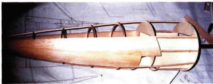
The sheeting is being glued to the formers. When all the sheeting except for the bottom is in place, remove the structure from the jig tube.
