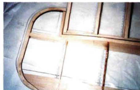
The aileron's counterbalance tips are made of two layers of lite-ply glued together.
