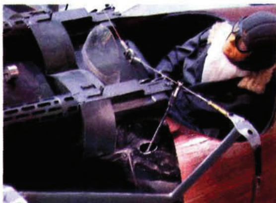
Above: the pushrod just ahead of the cockpit connects the aileron servo to the top wing's torque tube. Left: this is the attachment bracket connecting the aileron pushrod and the torque tube.
