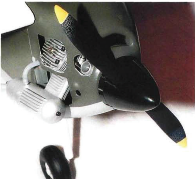
I used two O.S. .46FX 2-strokes in the prototype. The engines have been tilted to the 10-o'clock position to provide better muffler clearance.
