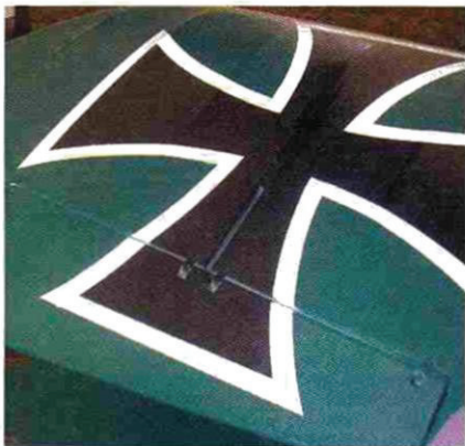
The ailerons use strap hinges, and the large slot in the wing is for the scale-like aileron control-horn linkage.
