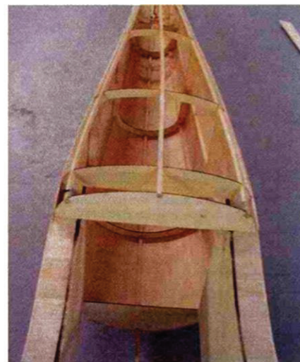
Here, the fuselage has been partially sheeted and slid off of the alignment pipe.
