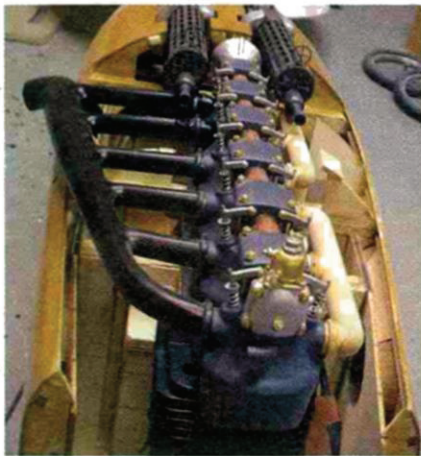
The dummy Mercedes engine covers the Zenoh G-62 nicely. The engine cowl has yet to be fitted into place.
