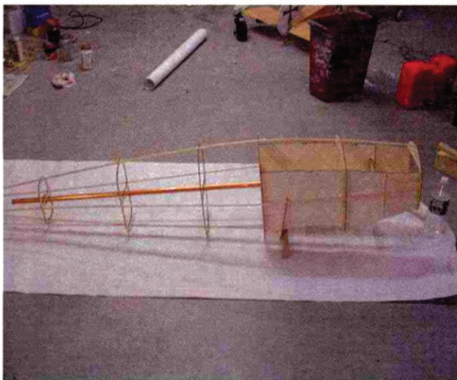
The basic fuselage is built around this box structure. The box and formers are then strung onto a length of copper pipe for alignment, and the stringers are added.
