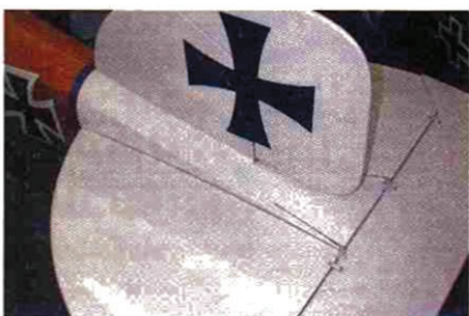
Completed tail surfaces are very scale-like and use pull-pull elevator cables.
