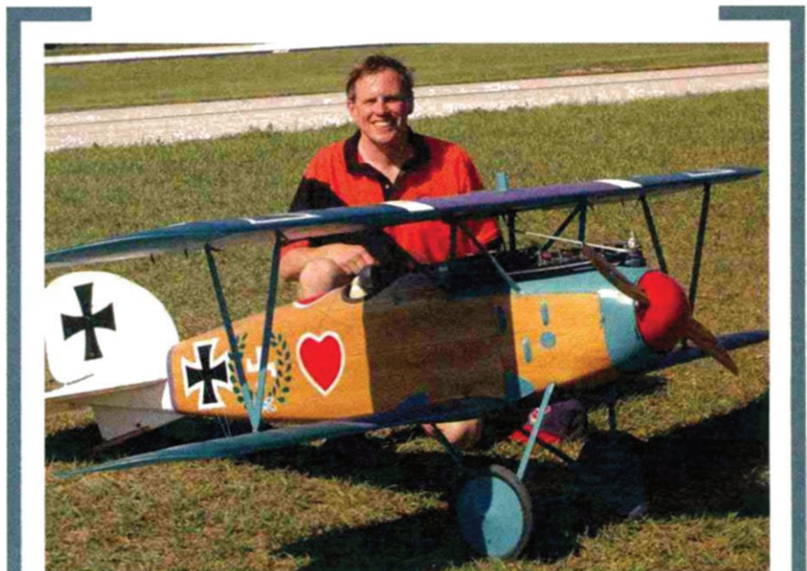
The completed dummy engine and engine cowl look very scale. Functional vents aid engine cooling.
