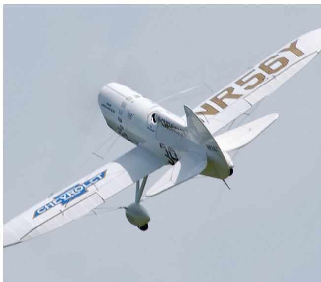
The Howard Ike is a great-flying design—aileron differential helps to eliminate adverse yaw.
