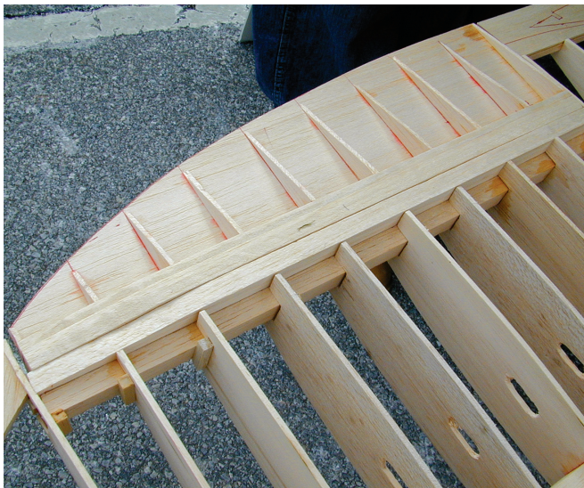
Here the aileron is being built as part of the wing structure. It will be separated and hinged back into place after the wing has been covered.
