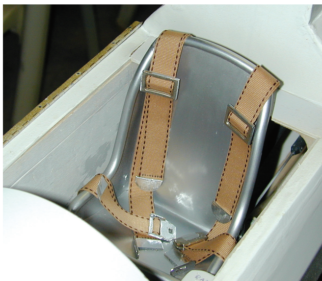
The removable pilot seat is held in place with magnets. The shoulder straps, seat belts and buckles all come from a fabric shop.
