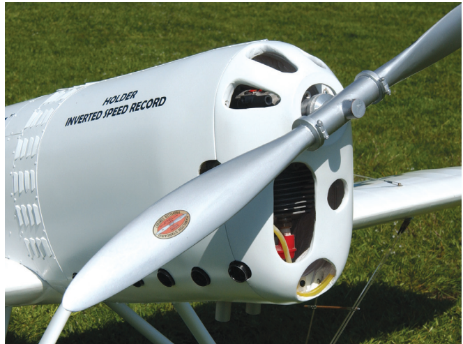
A scratch-built scale propeller adds a lot to the model's scale looks. The prop logo comes from Cal-Grafx.
