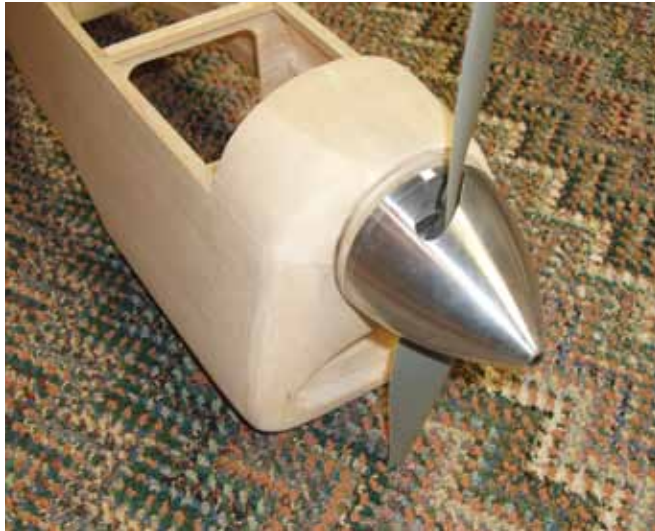
Here, you see the nose blocks shaped to blend into the spinner.
