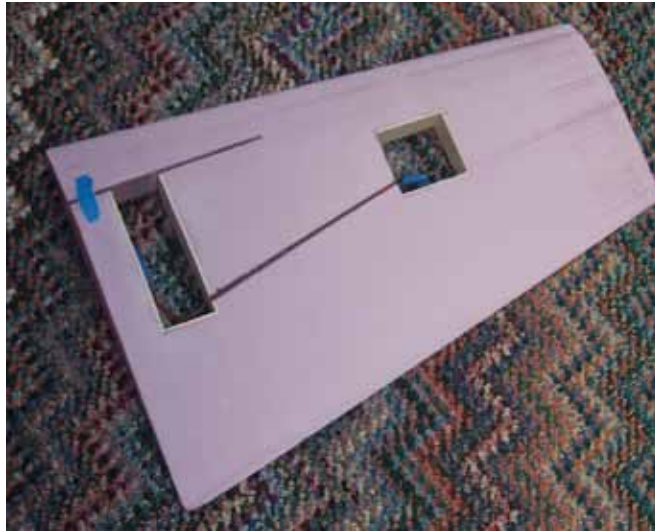
The wings are made out of foam cores cut with a hot wire. The tip and root templates are shown on the plans. Be sure to add the required wingtip washout.
