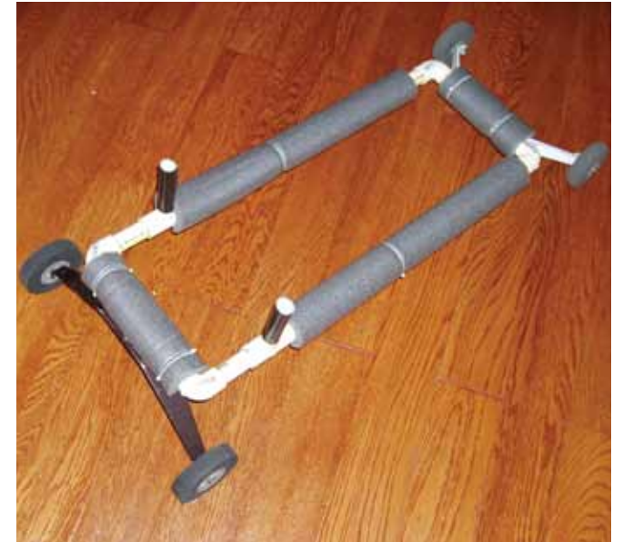
Here is the takeoff dolly. Hand-launching has proven difficult.
