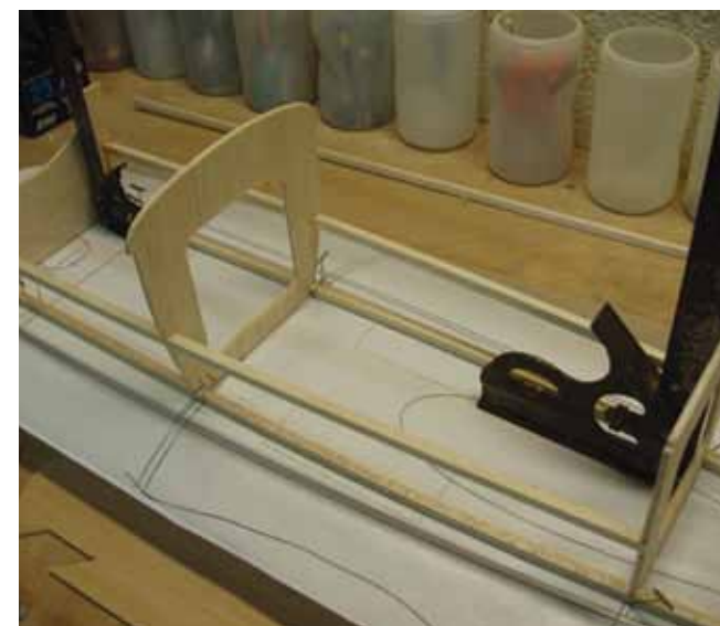
The fuselage is built upside-down over the plans. Start by pinning the longerons in place, and add the formers.
