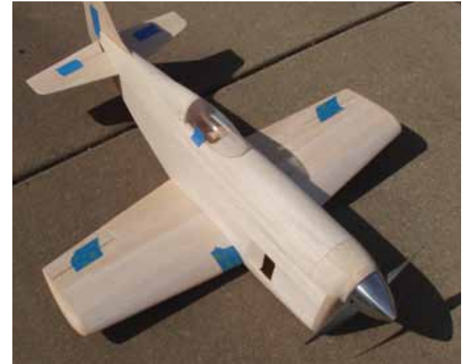
The final assembly, with the wings sheeted with balsa, shows how short those wings really are.
