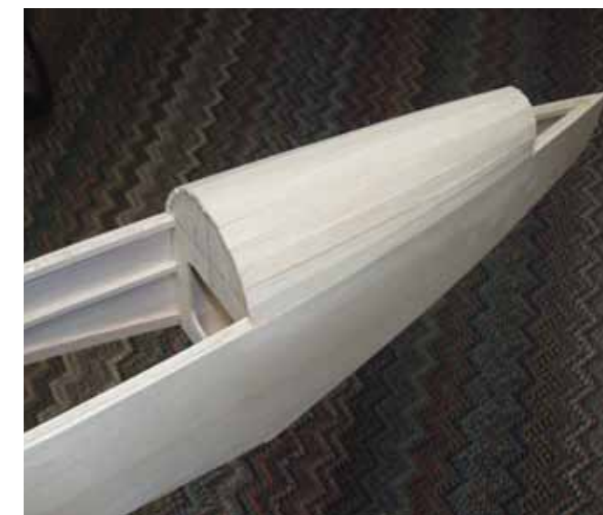
Sheeting the aft turtle deck gives the fuselage some shape.
