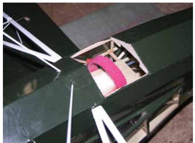
The battery is secured to the tray with hook-and-loop fasteners and a strap to prevent the battery from falling out. Also note the balsa plates under the cover at the rear center landing-gear struts.
