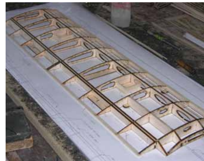
The finished wing panel will be removed from the board and sanded to final shape.
