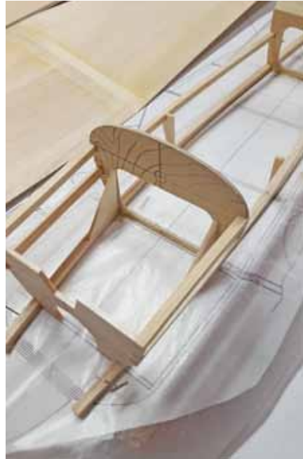
Make sure to install the formers and bulkheads properly. The firewall must be installed with side- and down-thrust offsets.
