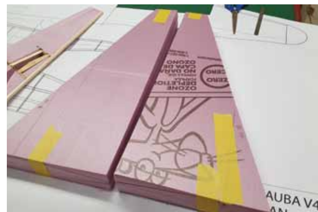
The wings are built with foam cores. I use pink insulation foam and cut them with the hot-wire technique. The templates for the root and tip airfoils are printed on the plans.
