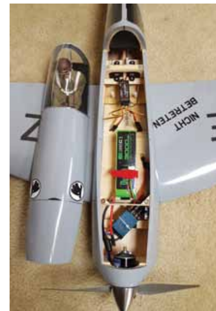
With the hatch cover (which includes the canopy section) removed, there is excellent access to the interior to allow you to get to the radio and power-system gear.
