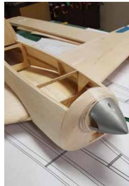
Here, the nose block and the front of the airplane has been shaped and sanded smooth. The spinner is used as a guide to get the nose block shaped properly.
