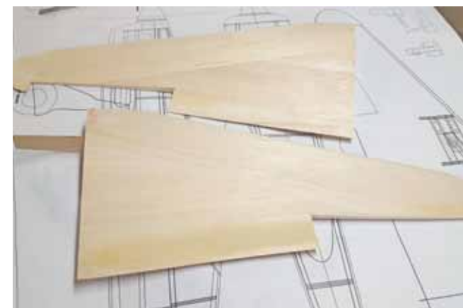
Here, the two wing panels have been sheeted with balsa. Notice the plywood joiner sticking out of the right panel.
