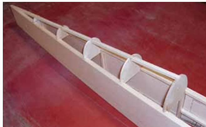
Here the turtle-deck formers and the top stringer have been added.
