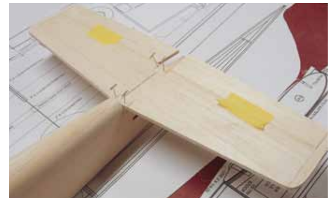
The tail surfaces are simple balsa sheet parts glued in place.
