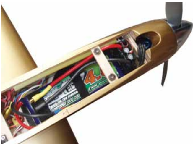
With the hatch cover removed, you have plenty of access to the model's radio gear and battery pack.
