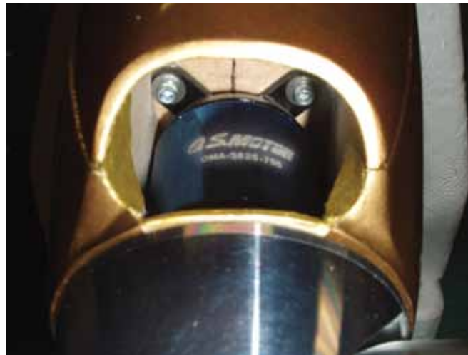
You can see the O.S. Engine brushless motor through the nose scoop, which provides plenty of cooling airflow.
