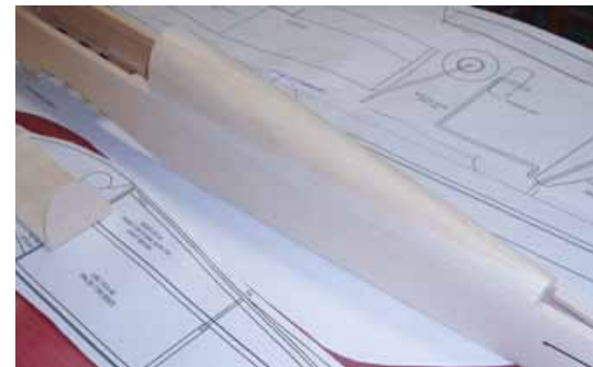
Sheet or plank the turtle deck with soft balsa, and let dry.
