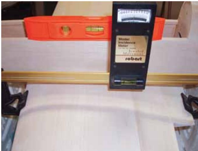
I used a Robart incidence meter to check the wing, making sure that it is properly aligned when set in place in the wing saddle.
