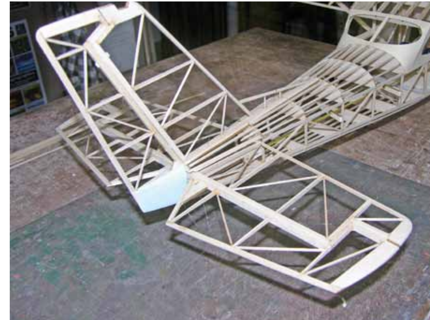
A section of the aft fuselage former is removed to allow the horizontal stabilizer to be fitted into the fuselage.
