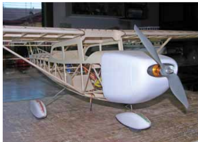
The vacuum-formed plastic cowl is built up and fitted onto the fuselage, then trimmed to fit the motor used.
