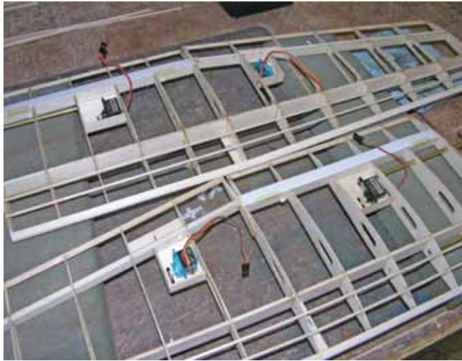
The flap and aileron servos are glued in place using silicone caulk.
