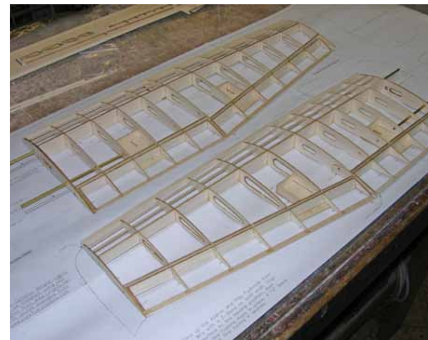
The flap and aileron assemblies are built directly over the plans, along with the main wing assembly. The brass joiner tubes are glued in place after the wings are sanded to final shape.
