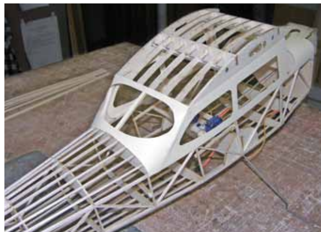
The window frames and fairings are made out of file-folder paper and glued in place around the cabin.
