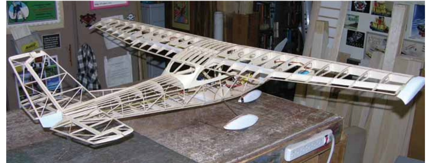
With all the framing and sanding done, the model is fully assembled to check for final fit and function while the internal components are still accessible.
