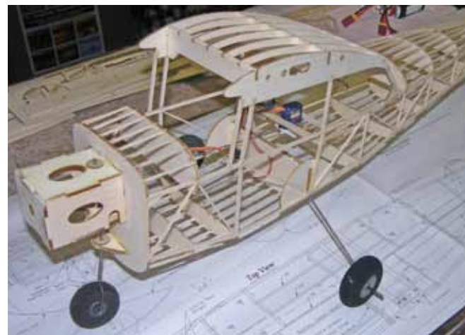
The fuselage assembly is finished with the addition of the servos, mounts, and all the top and bottom stringers.
