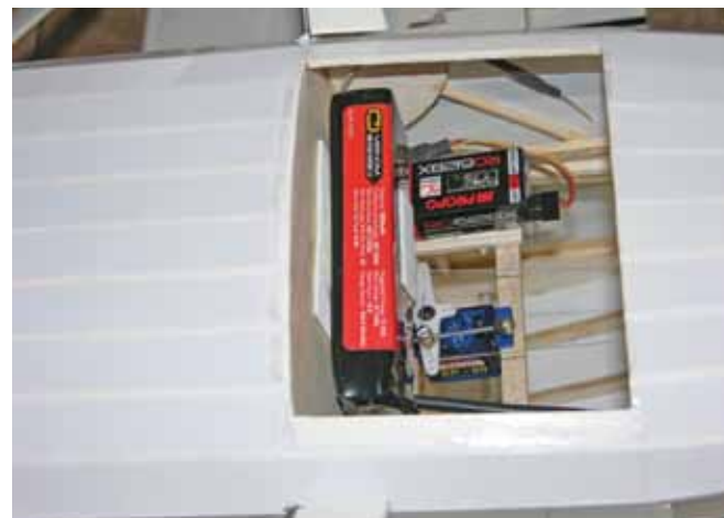
Access to the radio gear and battery is made through a hatch on the bottom of the fuselage.
