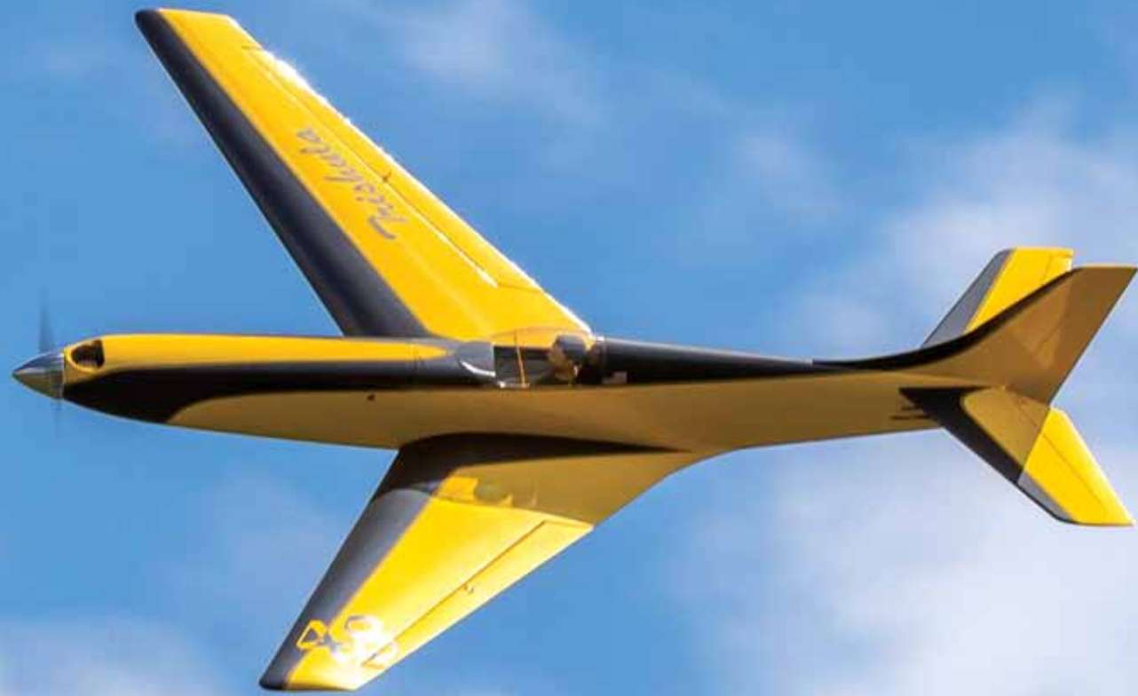
The Trishula has a unique appearance while flying. The forward-swept-wing planform takes a little getting used to.
