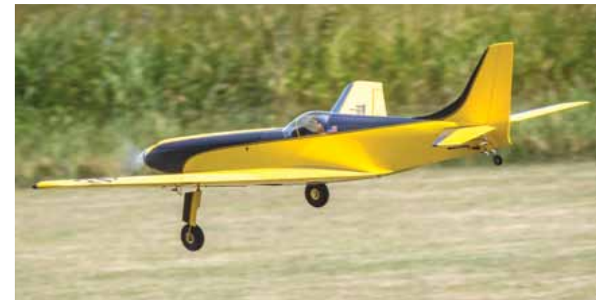
The Trishula is a tail-dragger, so you have to pay attention with the landings.
