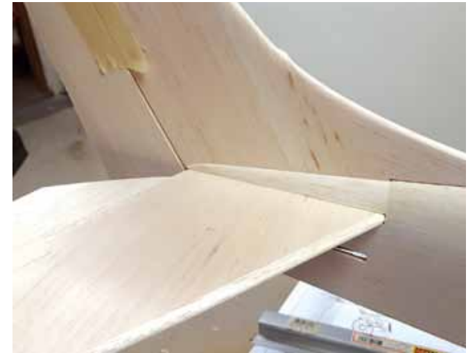
This shows the tail surfaces and fairing block installed and shaped to blend into the turtle deck.
