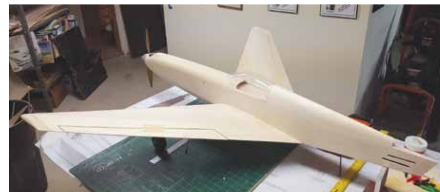
It's starting to look like a complete airplane. The fuselage sides have been joined at the tail, the turtle-deck sheeting has been applied, and the nose blocks have been installed and shaped.
