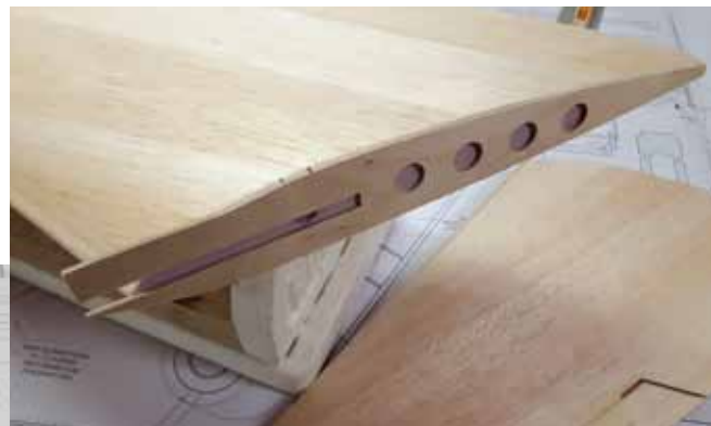
Before the wing panels are joined, glue the center rib into place.
