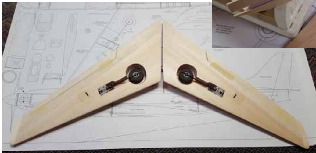
Here, you see the wing panels fully sheeted with balsa.
