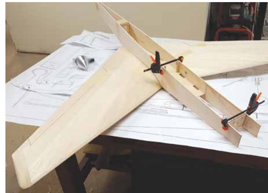
The basic fuselage structure is being assembled and placed on the wing assembly.
