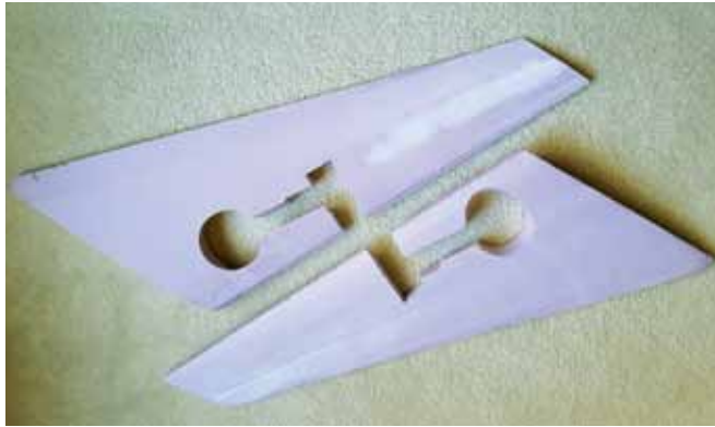
The wing cores for the Trishula are made out of pink foam. The airfoil templates are included on the plans.
