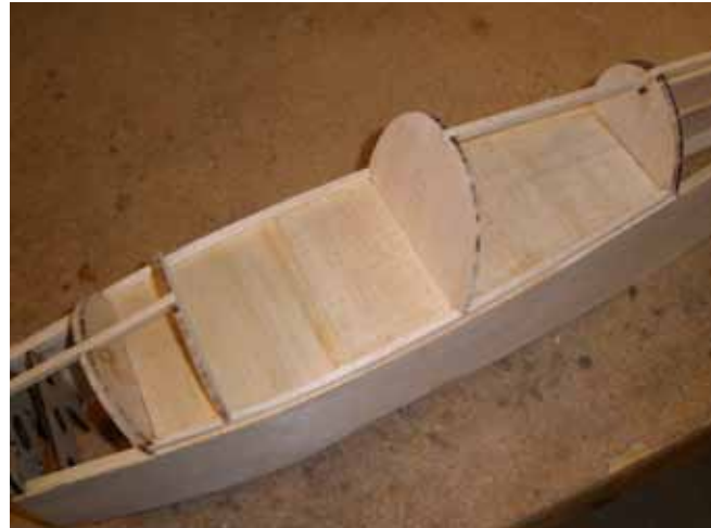
The main fuselage hatch is built on top of the assembled fuselage. There are angle-alignment template tools shown on the plans to properly install the upper formers.
