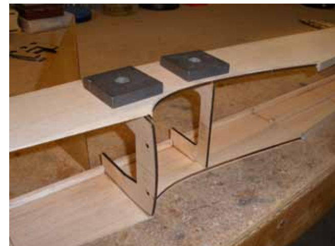
Start building the fuselage by gluing the top longeron in place, followed by these two formers. The weight holds them firmly in place until the glue dries. Make sure that the sides line up with each other.
