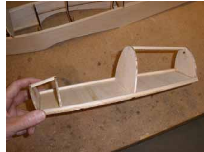
Here, the hatch-cover framework has been removed from the fuselage. It is then pinned to the workbench to keep it straight while applying the balsa sheeting.
