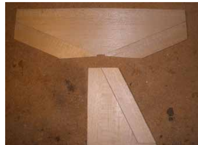
The tail feathers are made out of solid 3/16-inch balsa sheet. Simple straight lines make them quick to make.
