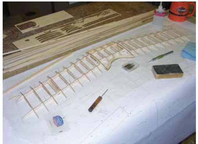
Here you see the top wing panels and center section being assembled over the plans.
