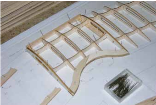
The top wing center section is built up directly over the plans. The trailing edge cutout is laminated from balsa to ensure a smooth transition when covered. The outer wing panels are framed up beginning with the rib and spar assemblies aligned over the plans and glued in place.
