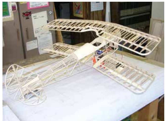
Here the airframe has been dry-fit together to check alignment and fit.
