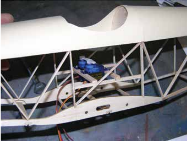
The large cockpit opening makes for easy access to the rudder and elevator servos when running in the pushrod and pull/pull cables.
