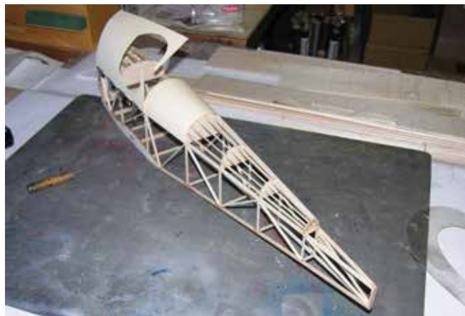
The fuselage is a typical structure with the side frames built flat on the plan's side view and then joined with the cross-pieces. Then the upper formers and the stringers are added.
