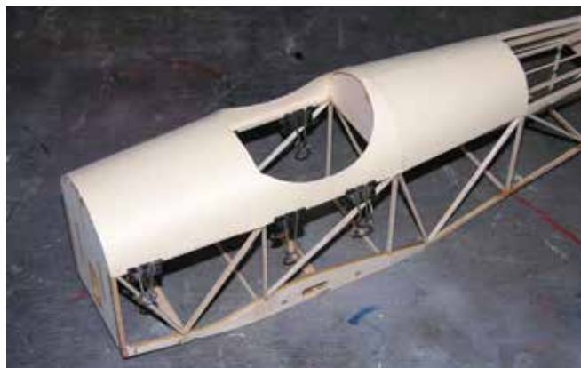
The cockpit fairings are made with file folder paper glued in place with Formula 560 canopy glue. The templates are shown on the plans.
