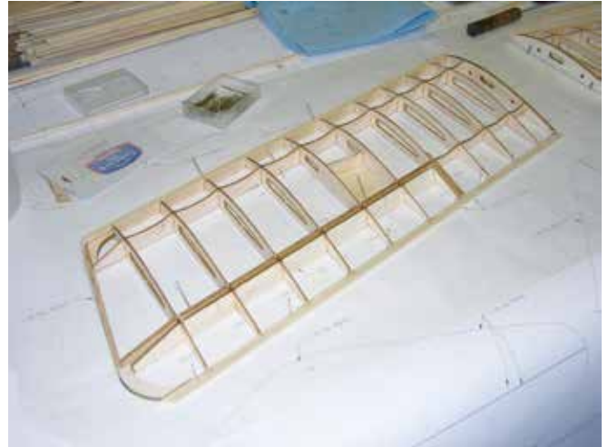
The wing panels are swept. Here is one of the bottom panels with the ailerons built as part of the panel and then later cut free.
