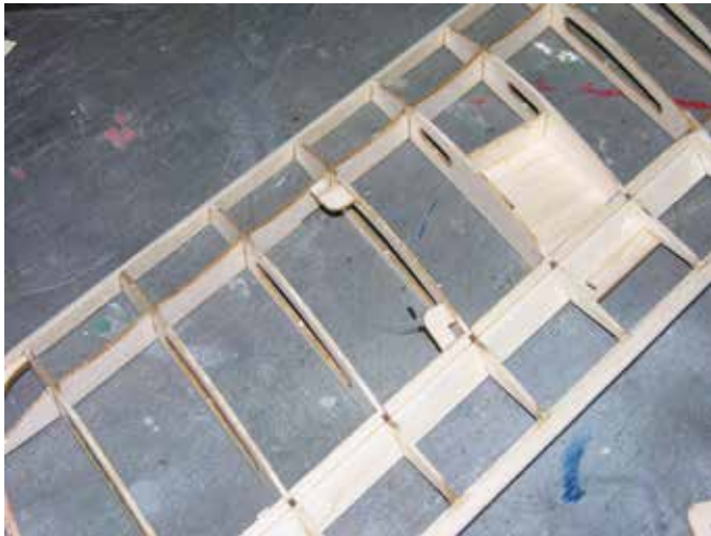
Here you see the aileron hinged into place plus the interplane strut supports and the servo attachment assembly glued in place.
