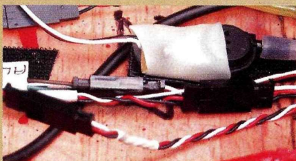
This is the barometric pressure sensor. Its function was to keep the model at a steady altitude.
