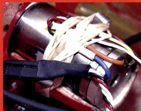
This is the alternator that supplies electrical power to all onboard systems. The engine's crankshaft provides the power to turn it.
