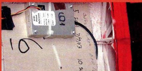
The GPS receiver is installed in the center wing section. Hook-and-loop fastener holds it in place.
