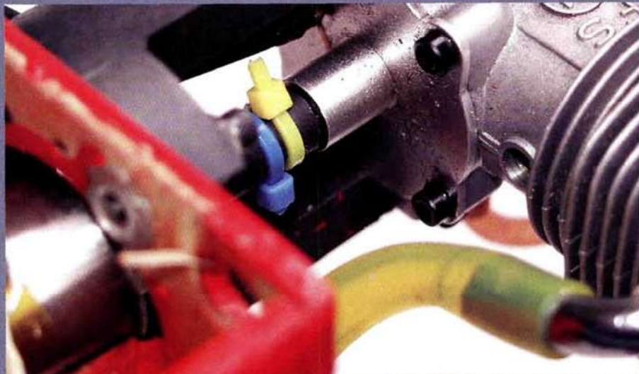
This is the alternator drive installed on the rear of the O.S. engine. A short length of vinyl tubing connects it to the alternator.
