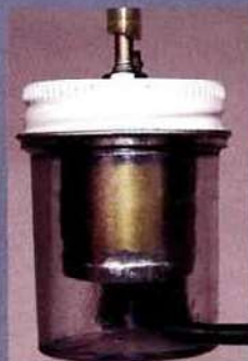
Maynard's home-made float chamber is pure simplicity: a plastic jar, some sheet brass and a no. 40 drill bit.
