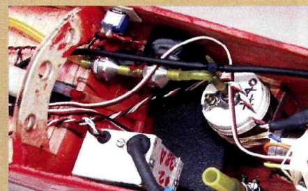
An overall view of the nose compartment. From left: on/off switch, backup battery, float chamber, C&H ignition module, carb and alternator. The throttle servo is mounted under the ignition module.
